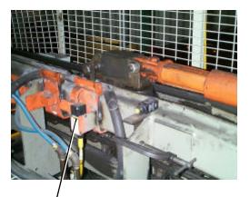
Limit Switch during actuation.
